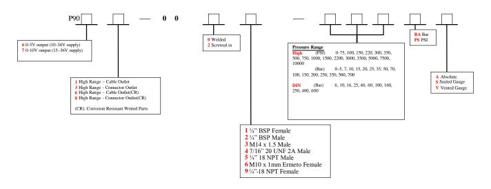
Examples: P90610002-7K5PSS = 0 to 5V output from 10 to 36V supply, cable outlet, welded  $\frac{1}{4}$ " BSP male port, 7500 psi sealed gauge
